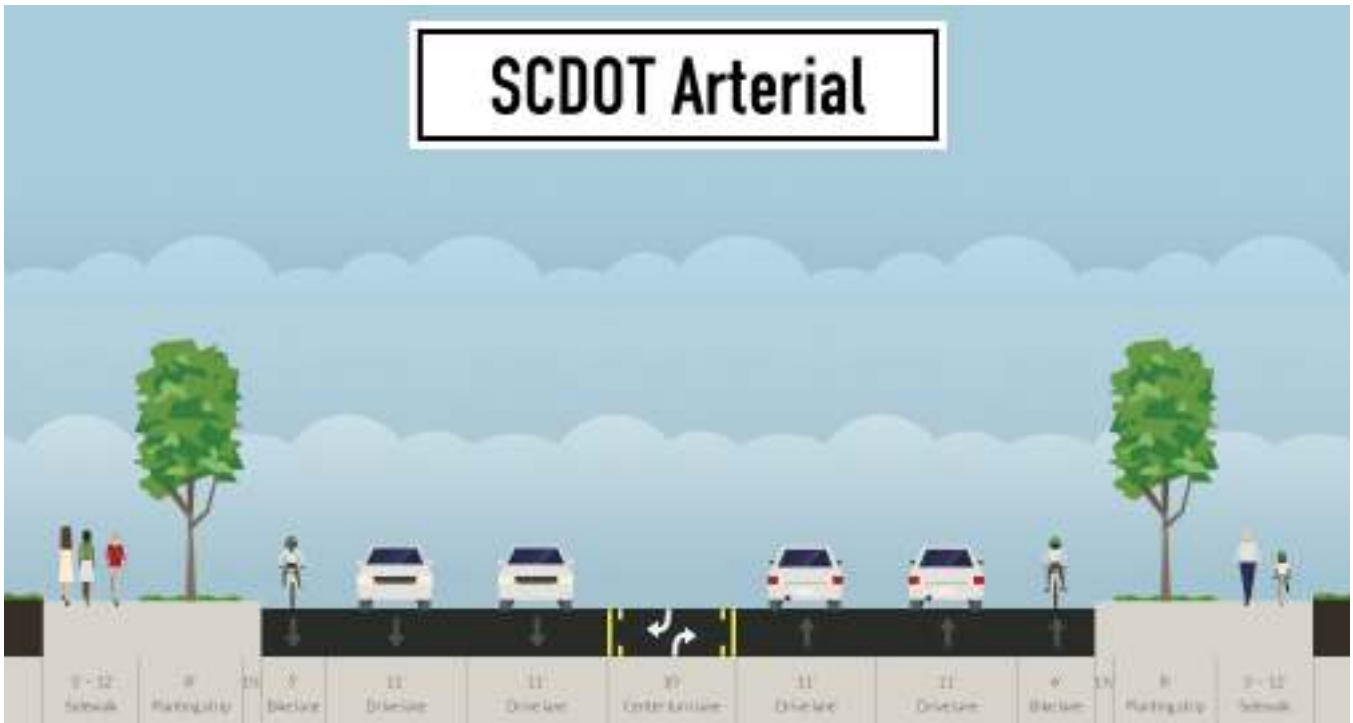
Conceptual section of South Carolina Department of Transportation arterial street
